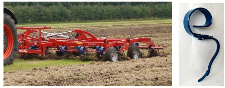
The spring loaded S-tine cultivator. A close up of the shape of the S-tines are displayed to the right (MARSK STIG Model 8).
